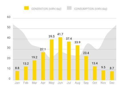
System Performance Assumptions: System Total losses: 13.5%, Inverter losses: 2.5%, Optimizer losses: 0%, Shading losses: 4.9%, Performance Adjustment: 0%, Output Calculator: System Advisor Model 2020.02.29.r2. Panel Orientations: 11 panels with Azimuth 103 and Slope 40, 3 panels with Azimuth 193 and Slope 40, 12 panels with Azimuth 283 and Slope 40.
